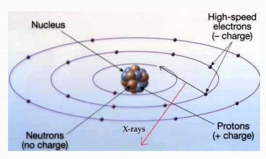
•A electron from an outer shell moves down to fill this vacancy and an x-ray is emitted.
